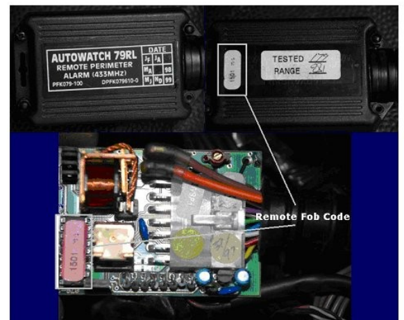
Fixed code found on very early Autowatch alarms uses 376-300 fobs
